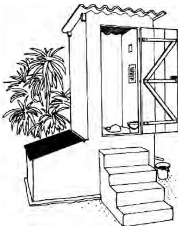
Figure 20 : Ecosan Toilet Source: ECOSAN Programme GTZ
